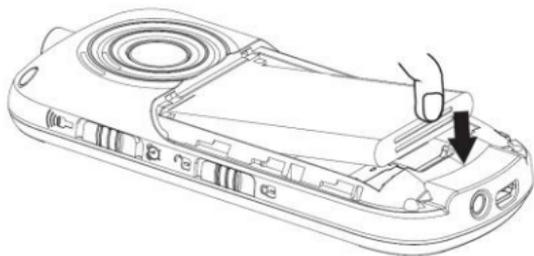
4. First After inserting the battery, slip cover. After the correct assumption is characteristic audible snap.
