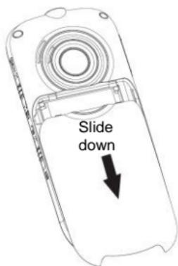
1. First When the phone is off, press the top cover and slide it in the direction shown in Figure
