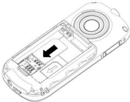
3. Insert the battery so that terminals + /- were directed to the top of the phone
